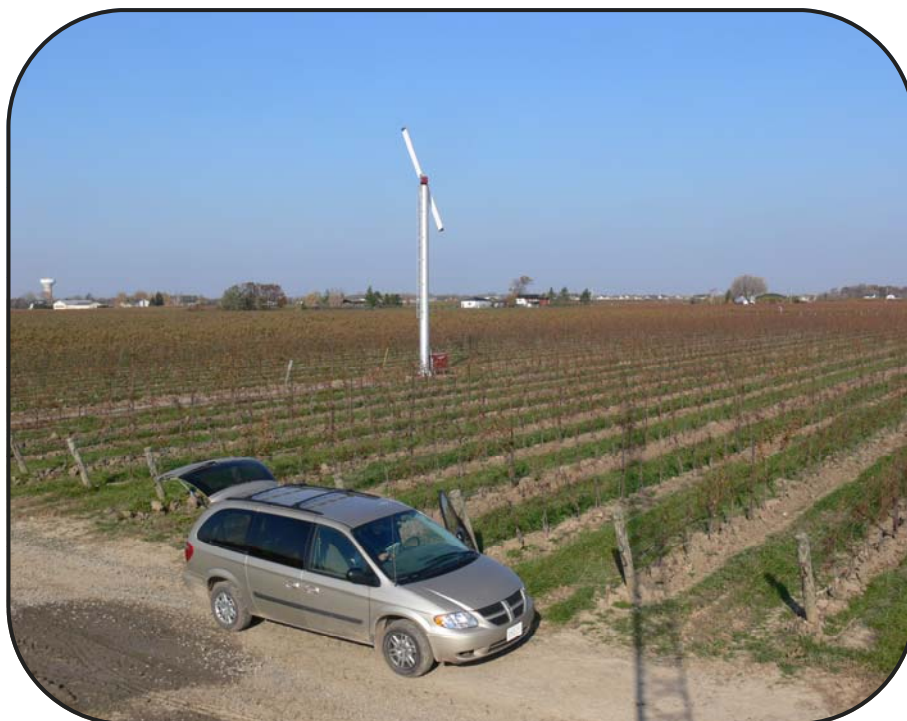
Figure 17. The location of the 20 m tower used to monitor air temperatures and wind speed/direction can be seen as a shadow in this picture and was 55 m (180 ft) southeast of the wind machine. The wind sensor was 10 m (33 ft) above ground on the tower, but because the wind machine fan hub was also at about the same height but blowing air 'downward', it did not appear to affect the wind sensor readings.
