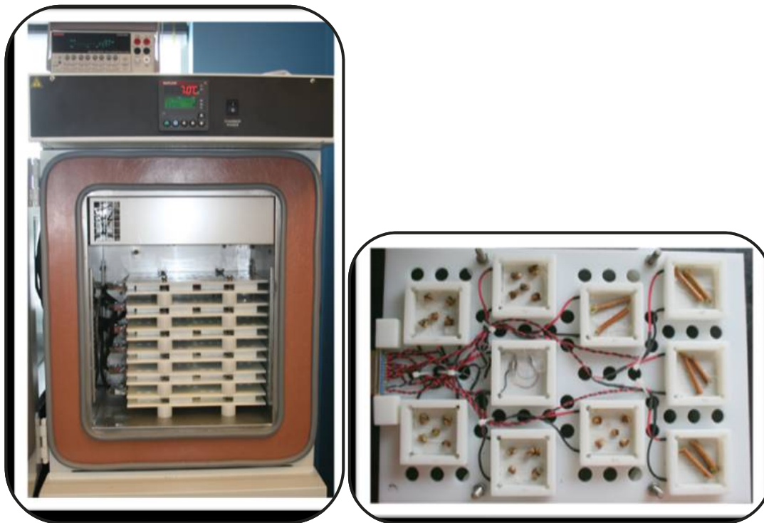
Figure 18. Differential thermal analysis (DTA) system programmable freezing chamber and loaded sample tray. Note the freezer is holding the maximum six sample trays per cycle. Cooling started at 4°C, then air temperatures were dropped slowly (4°C/h) over 12 hours to -40°C. Signals from the sample trays are transmitted to a multimeter (located on the top of the chamber), automatically converted to temperatures and loaded into an Excel spreadsheet.
