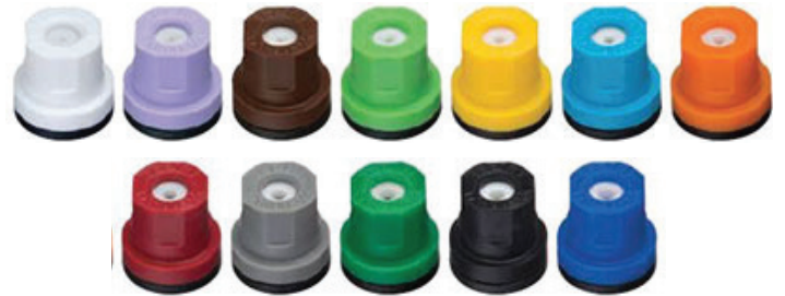
Figure 10. One-piece, color-coded, hollow-cone nozzles, each of which have their own flow rate. Flow rates increase from 0.053 gal/min (the white nozzle on the left, with the smallest orifice) to 0.49 gal/min (the blue nozzle on the right with the largest orifice) at the rated spray pressure of 40 psi.
